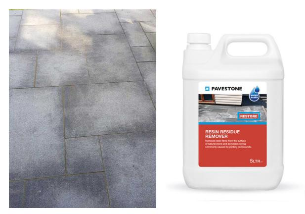
Jointing compounds can leave a residue of resin on paving that causes dark patches. The problem can be more noticeable on darker types of natural stone and is more likely to occur when paving is installed in hot weather.
