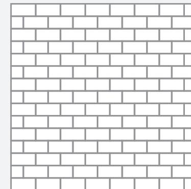
This laying pattern suitable for Alpha Antique and other mixed size block paving.
