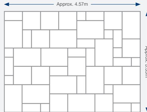
**Each Pack Contains:** 13 = 900 x 600mm, 13 = 600 x 600mm, 13 = 600 x 300mm, 9 = 290 x 290mm. 1 x 600 x 300mm not used in this pattern.
